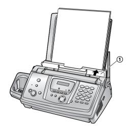
If the paper is not inserted correctly, readjust the paper, or the paper may jam.
